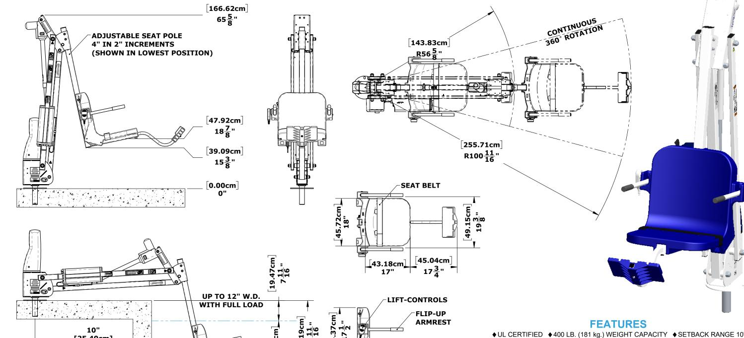
♦ UL CERTIFIED ♦ 400 LB. (181 kg.) WEIGHT CAPACITY ♦ SETBACK RANGE 10' TO 44" (26 - 111 cm) ◆ ADJUSTABLE SEAT POLE ◆ WATER DRAFT 12" ◆ 360° ROTATION ♦ FLIP UP ARMREST ♦ ALL STAINLESS STEEL CONSTRUCTION ♦ DURABLE POWDER COAT FINISH ◆ RECHARGEABLE BATTERY & WALL MOUNT CHARGER ♦ FIVE YEAR STRUCTURAL WARRANTY ♦ FIVE YEAR PRO-RATED ELECTRONICS WARRANTY
